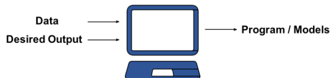
Figure 2: In traditional computer programming, you write a program to take in data and produce particular outputs. In ML, you provide input data and desired outputs to produce a “trained” model that can then be used for classification or prediction when given new inputs..
